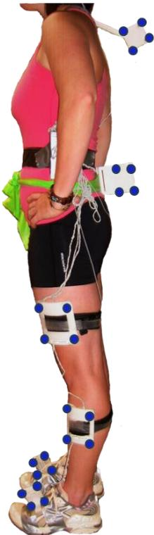
**Figure A.1: Marker cluster set-up and configuration. Blue dots represent individual IRED markers.**
