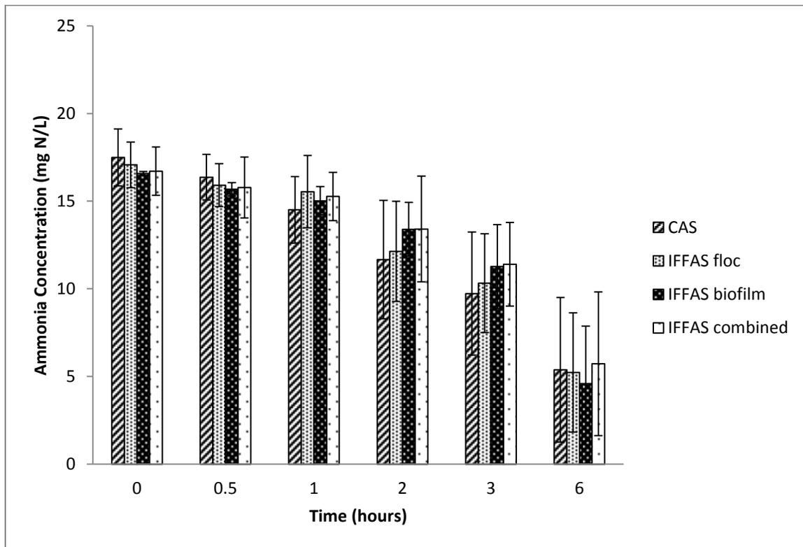
**Figure 3. Ammonia removal (mg N/L) observed in CAS, IFFAS flocc, IFFAS biofilm, and IFFAS combined flocc and biofilm for batch experiment (6 hours) run under aerated conditions. All data collected from four replicates with standard deviations shown with error bars.**
