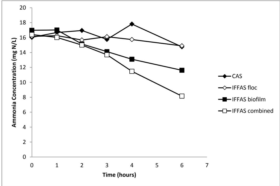
**Figure 1. Ammonia removal (mg N/L) observed in CAS, IFFAS floc, IFFAS biofilm, and IFFAS combined flocs and biofilm for initial batch experiment (6 hours) run under non-aerated conditions.**
