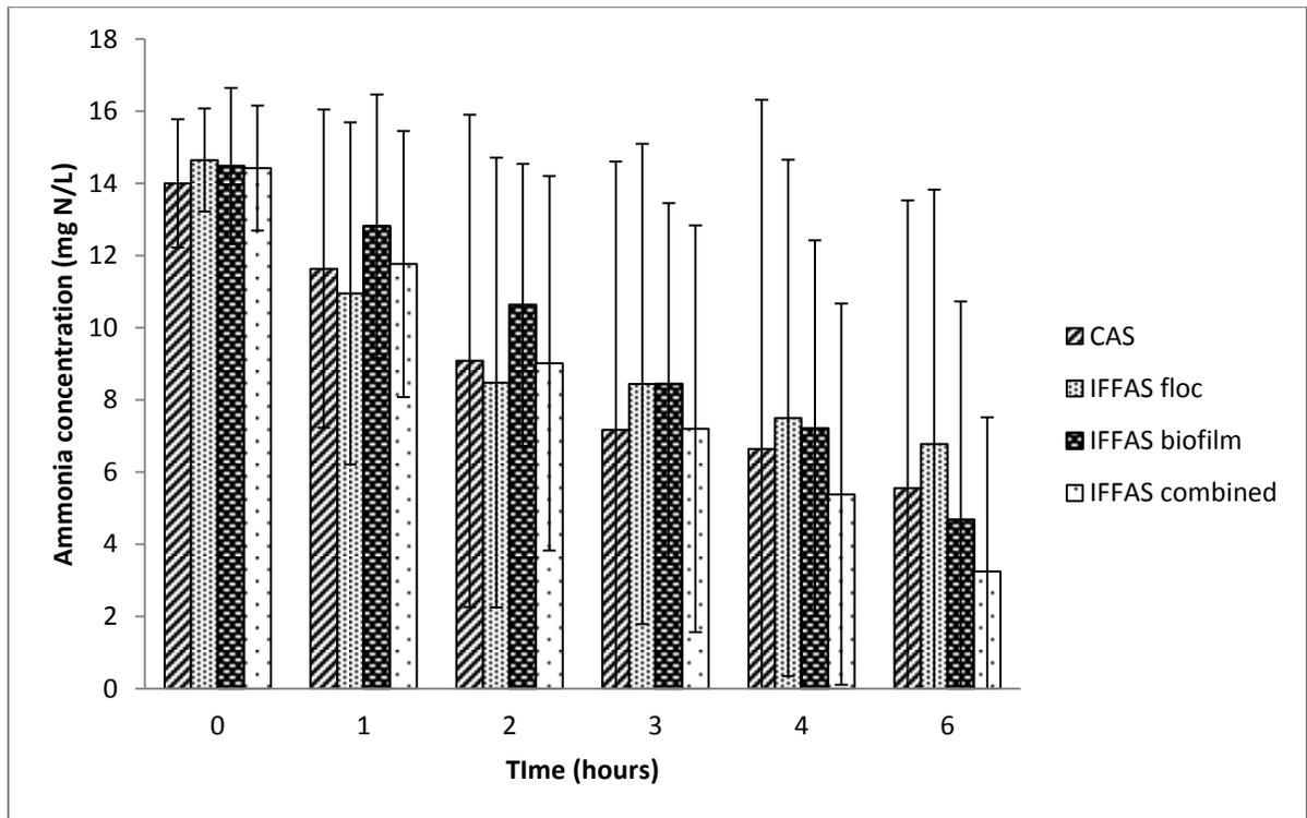
**Figure 2. Ammonia removal (mg N/L) observed in CAS, IFFAS floc, IFFAS biofilm, and IFFAS combined flocs and biofilm for batch experiment (6 hours) run under non-aerated conditions. All data are presented in triplicate with standard deviations shown with error bars.**
