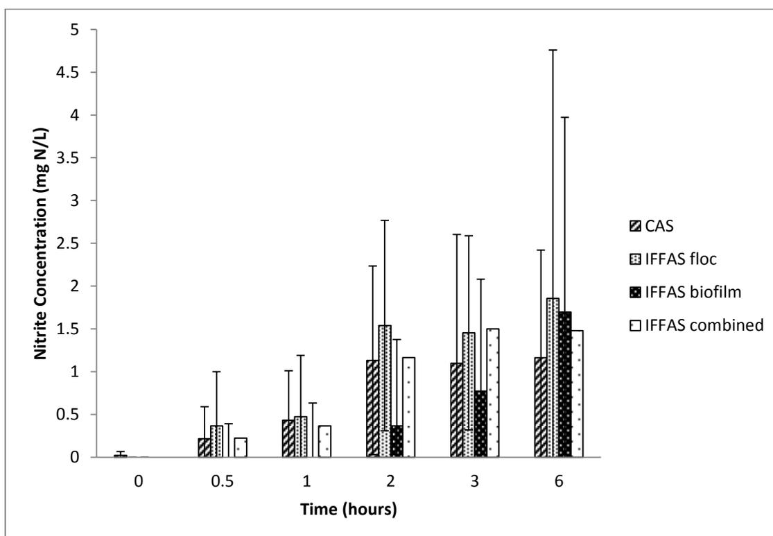
**Figure 4. Nitrite concentrations (mg N/L) observed in CAS, IFFAS flocc, IFFAS biofilm, and IFFAS combined floccs and biofilm for aerated batch experiment (6 hours). All data collected in triplicate with standard deviations shown with error bars.**
