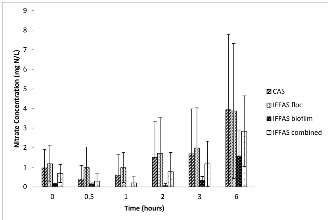
**Figure 5. Nitrate concentrations (mg N/L) observed in CAS, IFFAS floc, IFFAS biofilm, and IFFAS combined flocs and biofilm for aerated batch experiment (6 hours). All data collected in triplicate with standard deviations shown with error bars.**
