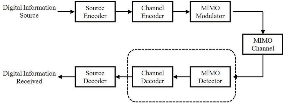
Figure 1.3: A basic MIMO system diagram.
