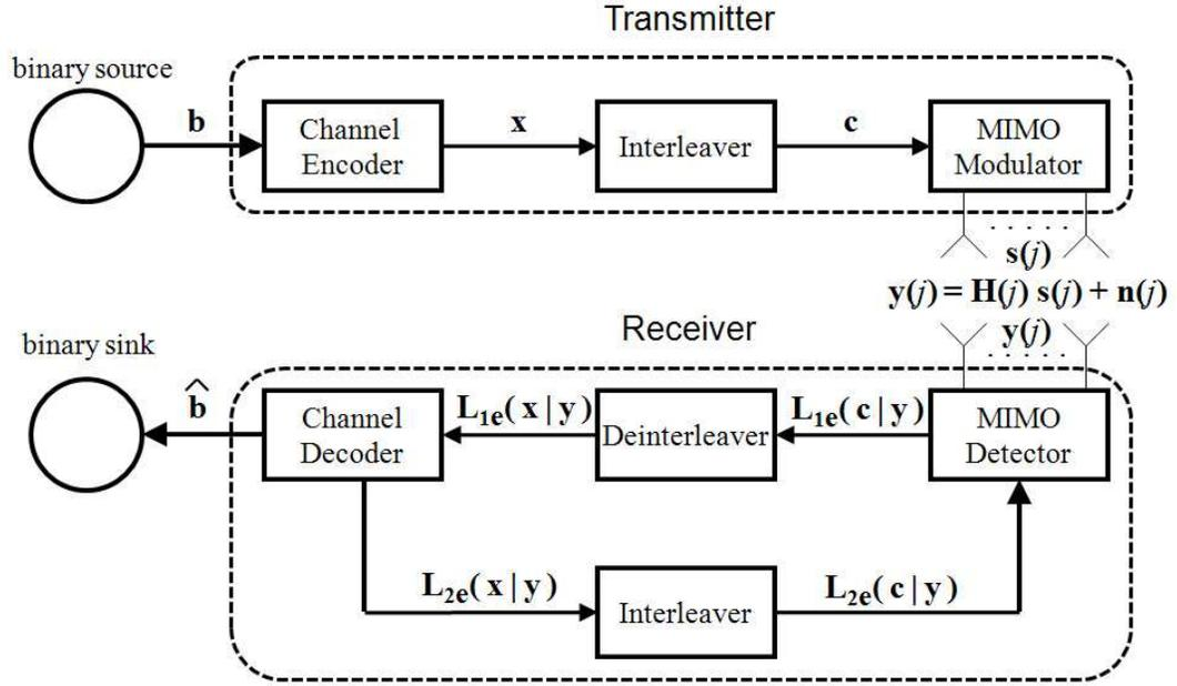
Figure 2.2: Iterative Joint Detection and Decoding System Model.
