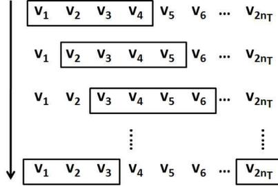
Figure 4.3: Illustration of Window Shifting Detection.
