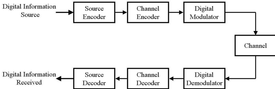
Figure 1.2: The basic elements of a digital communication system.
