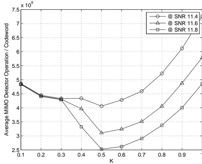
Figure 3.1: Complexity analysis of various choices of radius in  $4 \times 4$  V-BLAST LSD IJDD MIMO system employing WiMAX A Code, 16-QAM, and interleaver size of 6912.
