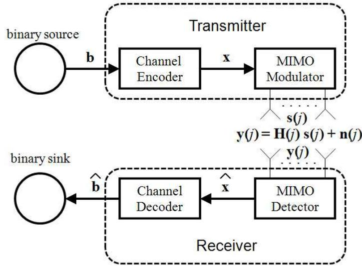
Figure 2.1: MIMO system model with a serial concatenated receiver.
