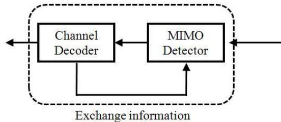
Figure 1.4: Abstract framework of iterative joint detection and decoding in MIMO systems.
