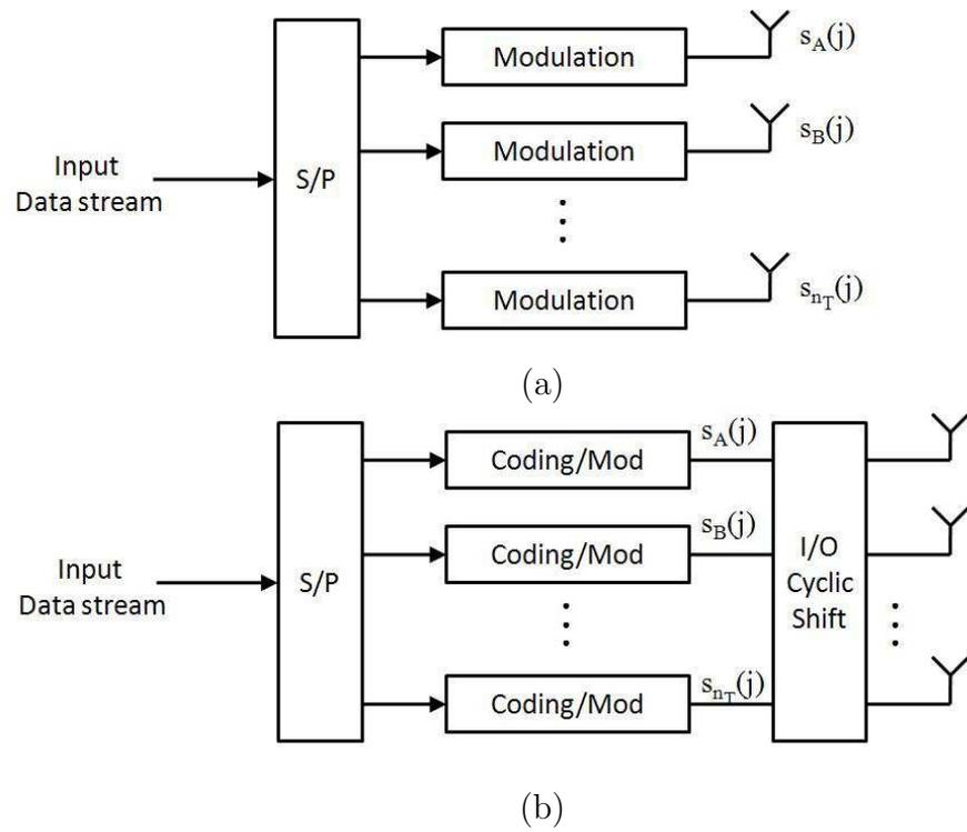
Figure 2.3: (a) V-BLAST encoder (b) D-BLAST encoder.
