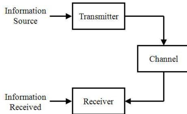
Figure 1.1: Basic communication system.
