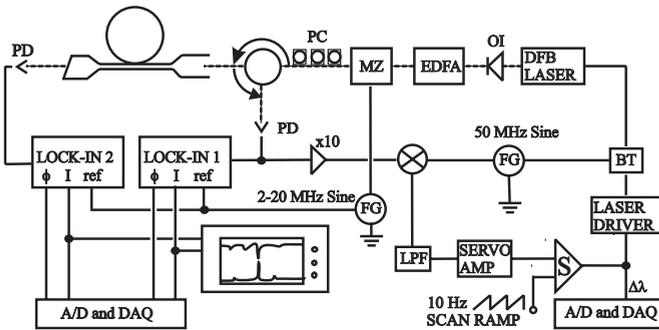
FIG. 1. Setup showing the Pound-Drever-Hall scheme. Distributed feedback laser (DFB); optical isolator (OI); erbium-doped fiber amplifier (EDFA); Mach-Zehnder amplitude modulator (MZ); polarization controller (PC); photodiode (PD); function generator (FG); low-pass filter (LPF); bias-T (BT).
