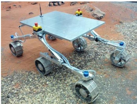
Figure 4 HDPC Original Setup (Produced by ETH)
