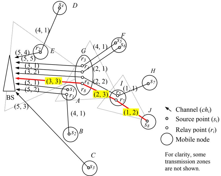
**Figure 4.7: Channel assignment for the virtual points corresponding to the scenario in Figure 4.1**
