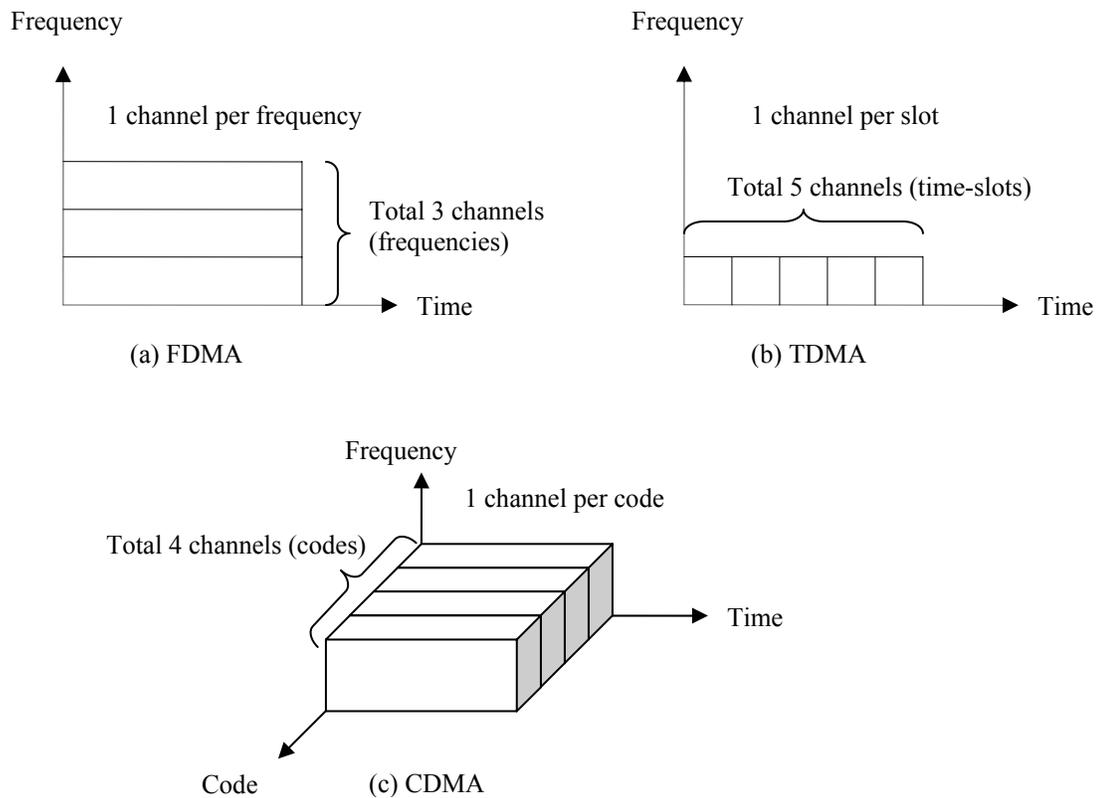
**Figure 3.2: Three multiple access techniques: a) FDMA, b) TDMA and c) CDMA**
