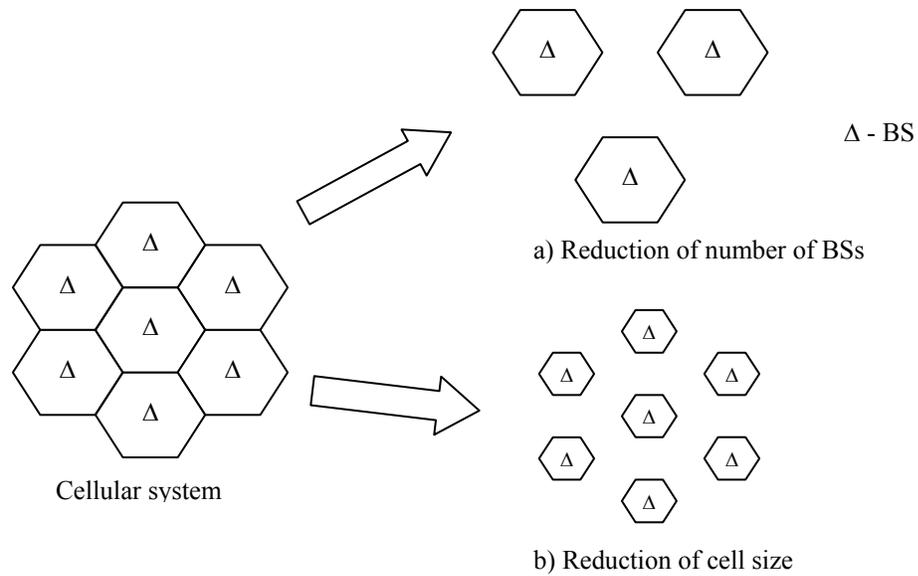
**Figure 1.3: Reduction of number of BSs and cell size of a cellular system**
