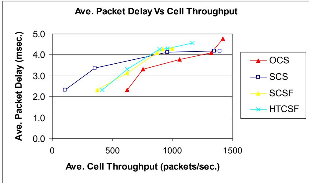
Figure 5.12: Packet Delay versus Cell Throughput
