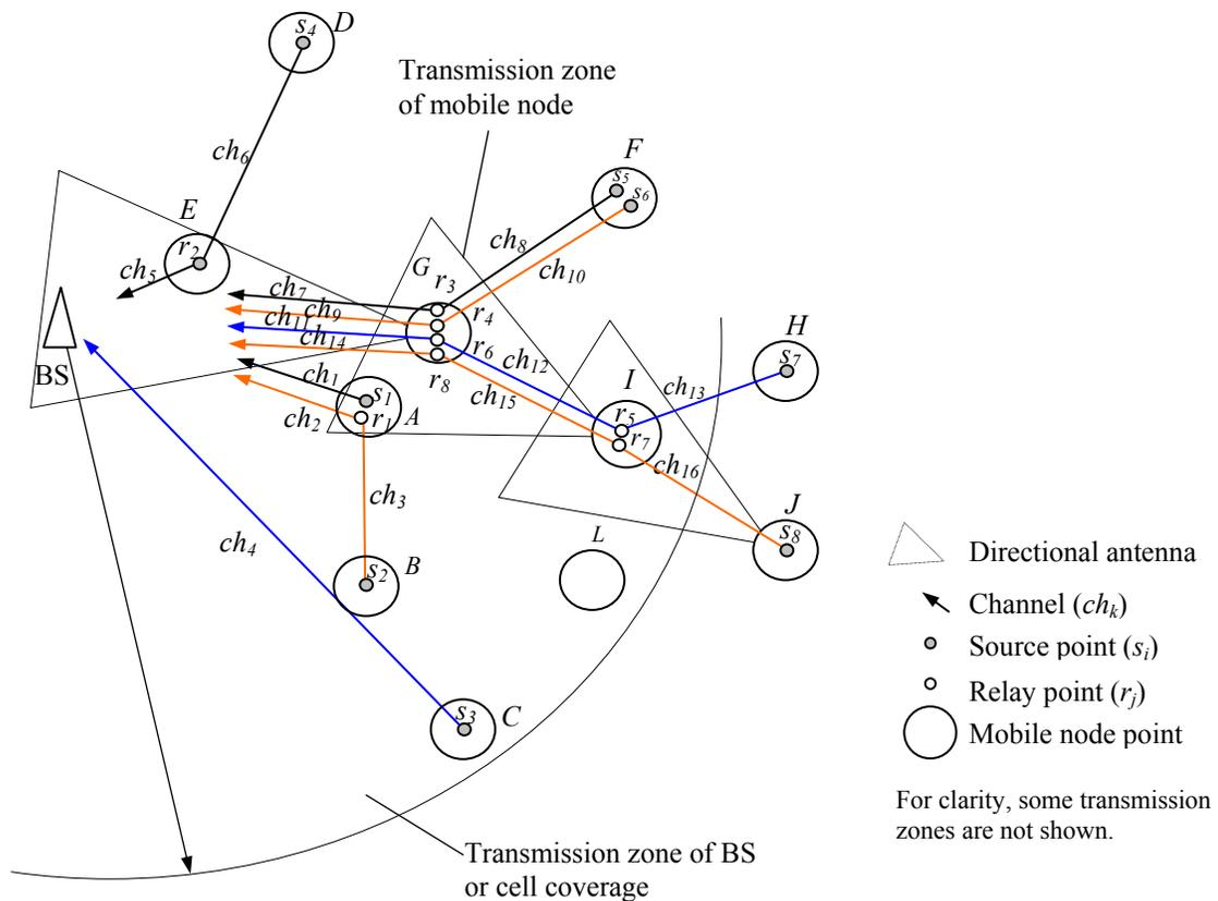
Figure 4.1: Topology and channel assignment in a MCN with directional antennas
