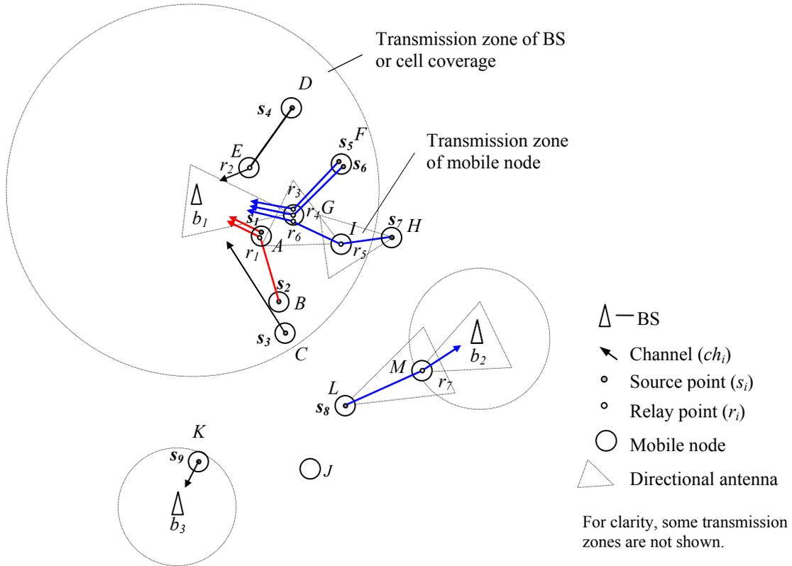
**Figure 3.5: Topology in a MCN with directional antennas**
