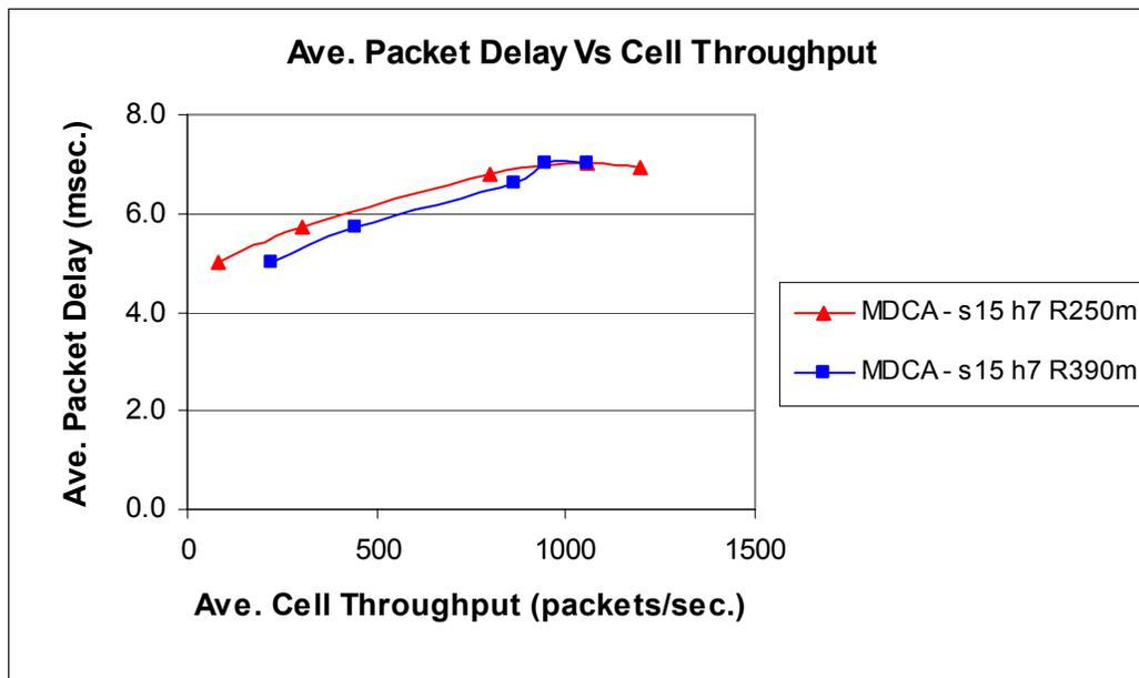
Figure 4.13: Packet Delay versus Cell Throughput (Scenario 2)
