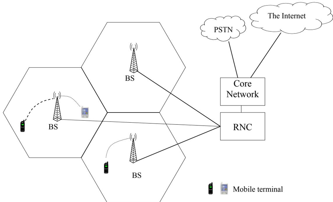
**Figure 1.1: System architecture of a 3G cellular system**
