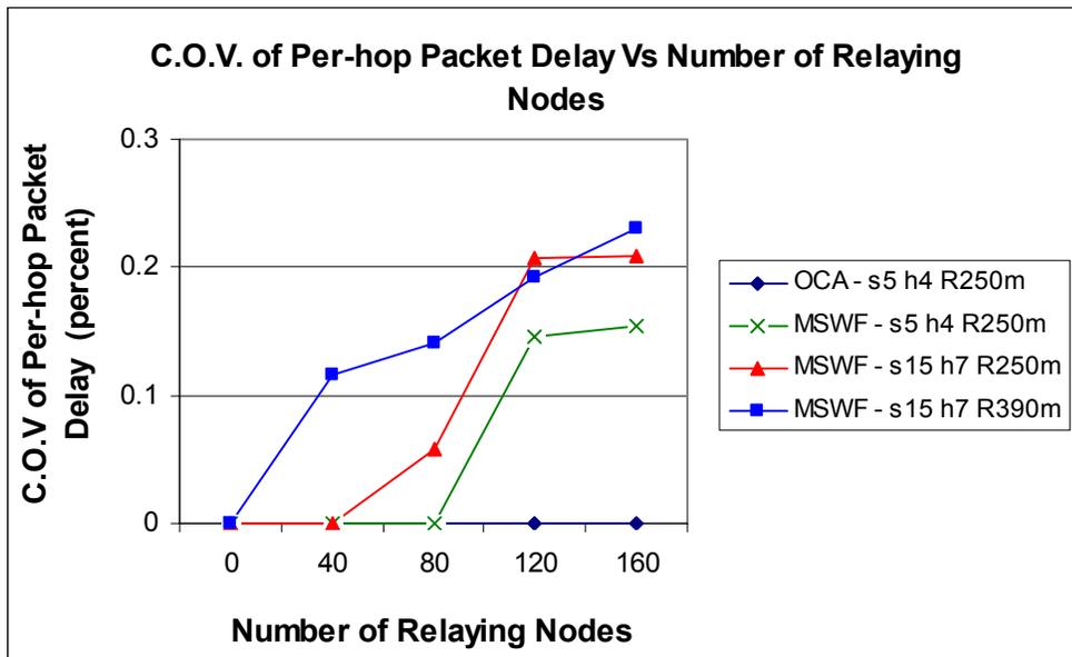
Figure 4.10: C.O.V. of Per-hop Packet Delay (Scenarios 1 and 2)
