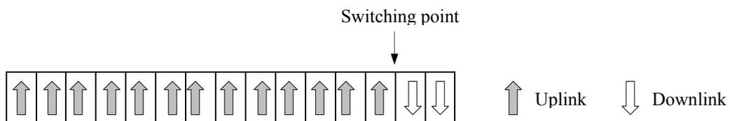
**Figure 2.4: A switching point in a TDD CDMA transmission frame**
