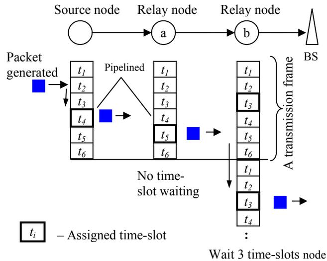
**Figure 4.2: Time-slot waiting time (relaying delay) at relaying nodes on relaying path**
