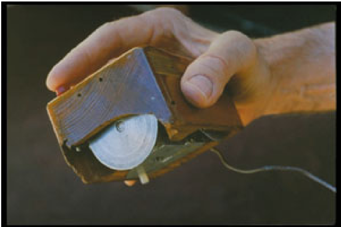
Figure 2.1: Douglas Engelbart’s prototype mouse design [12].
