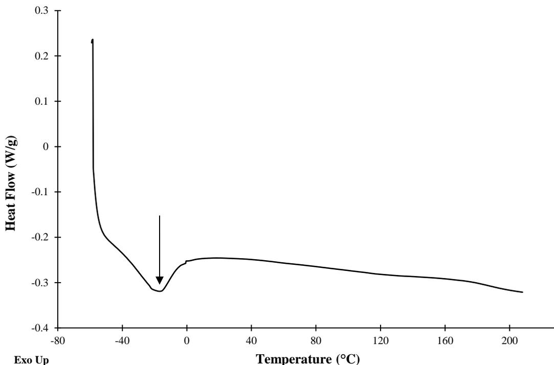
**Figure 4.1: Second heating DSC scan of P(VC<sub>12</sub>ImBr). The arrow marks the peak indicating the  $T_m$  of P(VC<sub>12</sub>ImBr).**
