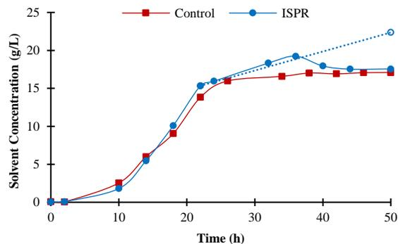
**Figure 4.7: Concentration levels of total solvents (*n*-butanol, acetone, and ethanol) in the control and ISPR ABE fermentations, where the solid lines represent the aqueous solvents, and the dashed line and open symbol represent the equivalent concentration absorbed by P(VC<sub>12</sub>ImBr) in the ISPR fermentation.**
