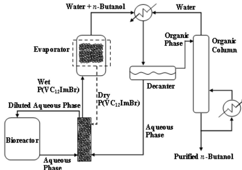
**Figure 4.8: Proposed layout of continuous ABE ISPR fermentation using  $P(\text{VC}_{12}\text{ImBr})$  with one distillation column for  $n$ -butanol purification.**
