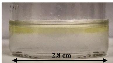
**Figure 4.11: Recovered liquid from equilibrated P(VC<sub>12</sub>ImBr) through experimental procedure.**
