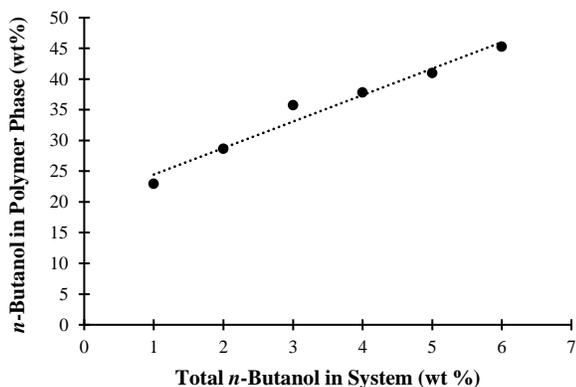
**Figure 4.10: Content of *n*-butanol absorbed by P(VC<sub>12</sub>ImBr) at equilibrium in relation to the total *n*-butanol content of the system.**
