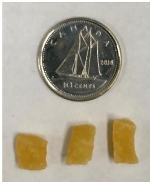
**Figure 3.1: Pieces of P(VC<sub>12</sub>ImBr) that were synthesized and formed for use in this work next to a dime for size reference.**
