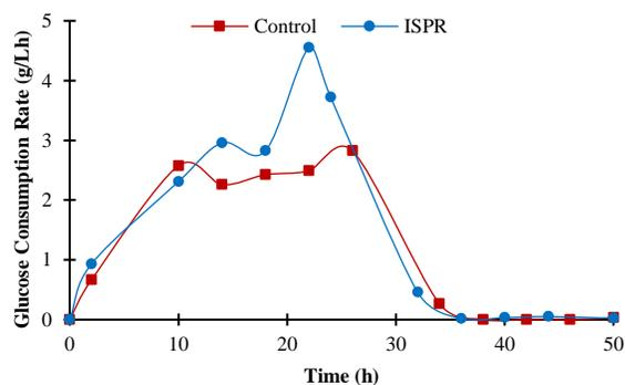
**Figure 4.6: Instantaneous glucose consumption rates for control and ISPR ABE fermentations.**
