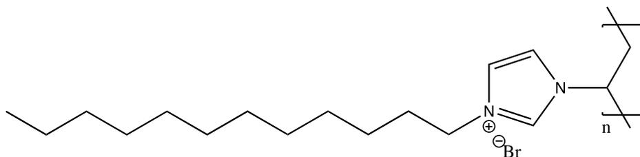
**Figure 2.2: Chemical structure of P(VC<sub>12</sub>ImBr)**
