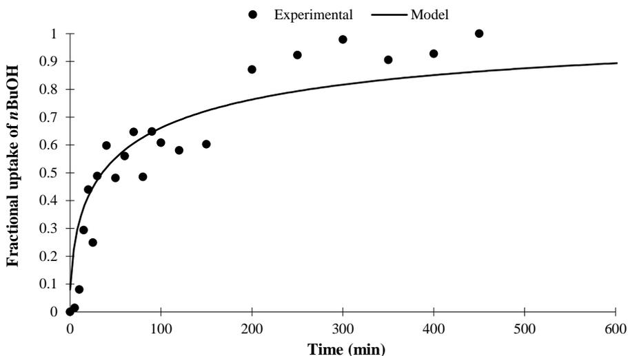
**Figure 4.2: Experimental and model time course of the uptake of *n*-butanol by 5% (w/v) P(VC<sub>12</sub>ImBr) in 1 L of a 2 wt% concentration *n*-butanol solution.**
