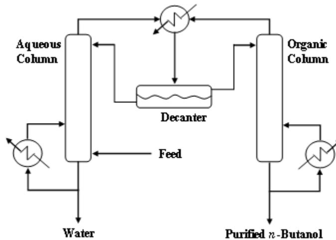
**Figure 2.1: Flow of *n*-butanol purification process by distillation**
