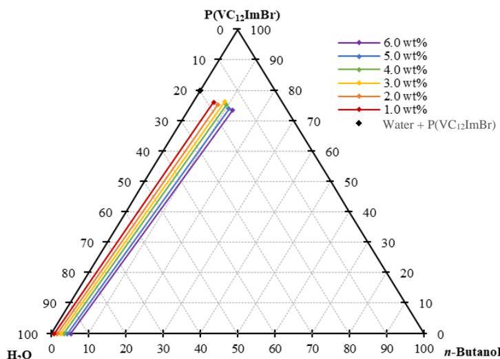
**Figure 4.9: Ternary diagram (in wt%) constructed by experimental data of the water + *n*-butanol + P(VC<sub>12</sub>ImBr) system at equilibrium with a consistent polymer mass fraction at 5% (w/v) and varying initial *n*-butanol concentration.**
