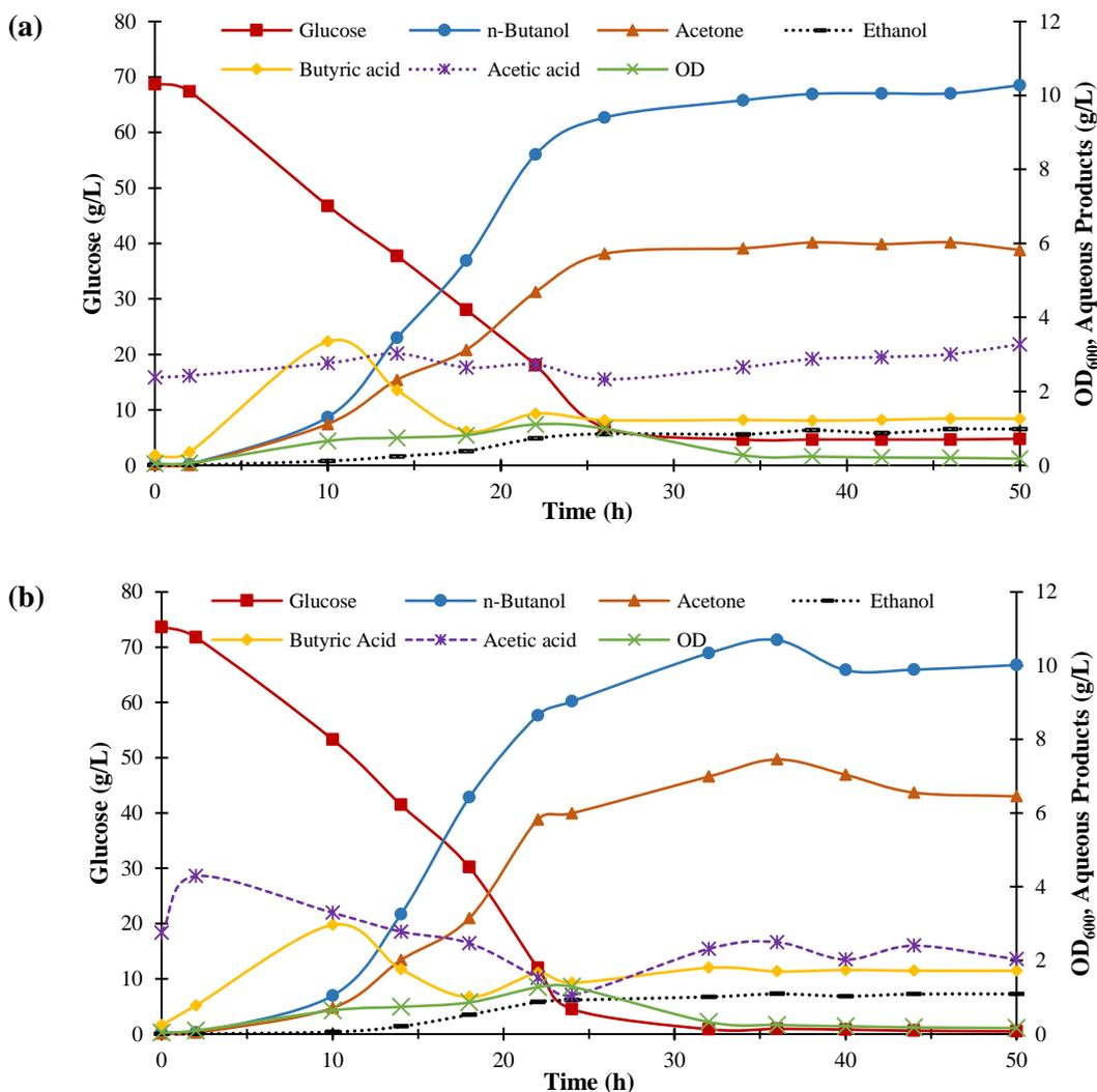
**Figure 4.5: Kinetics of batch ABE fermentations by *C. acetobutylicum*; (a) control fermentation with no ISPR; (b) ISPR fermentation where contact of fermentation broth with 5% (w/v) P(VC<sub>12</sub>ImBr) was initiated at 18 hours.**
