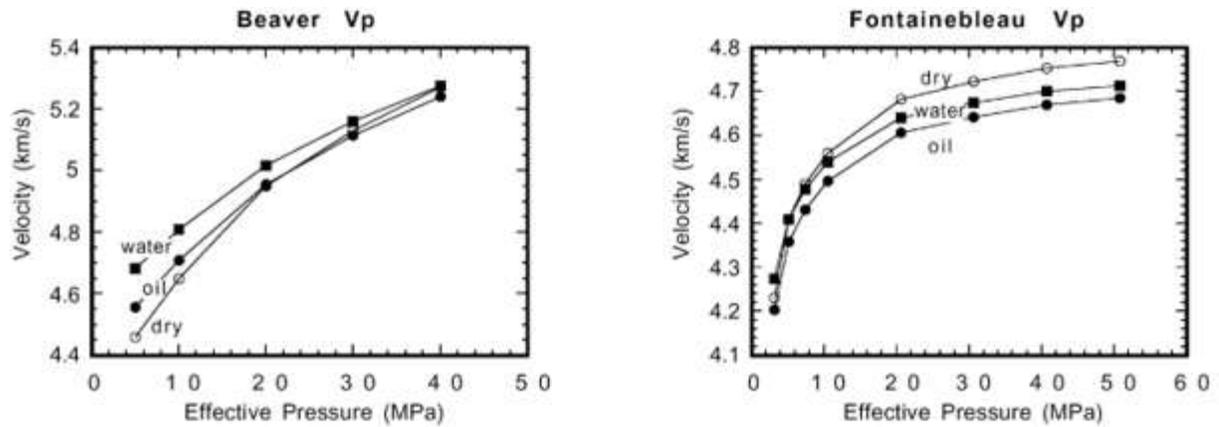
Figure 5: Velocity VS Effective pressure applied on Beaver sandstone (6% porosity on left) and Fontainebleau sandstone (15% porosity on right) for varying fluids used to penetrate the porous space of the materials (Mavko, 2017).
