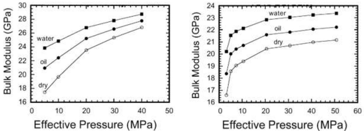
Figure 4: Bulk Modulus for porous sandstones VS the effective pressure applied. Different fluids with different densities and bulk moduli. Beaver sandstone, with a porosity of 6%, is on the left, while Fontainebleau sandstone, with a porosity of 15% is on the right (Mavko, 2017).
