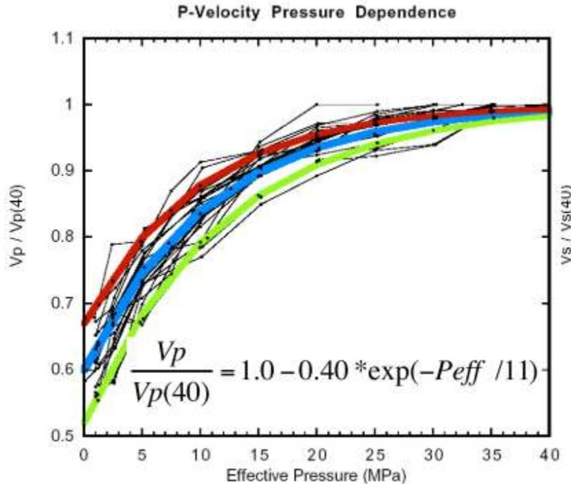
Figure 3: P-wave dependence on the effective pressure exerted on a rock samples for sample data. Three potential exponential models are drawn to show potential models to describe the relationship, while the average relationship is described mathematically with an exponential model. (Mavko, 2017)
