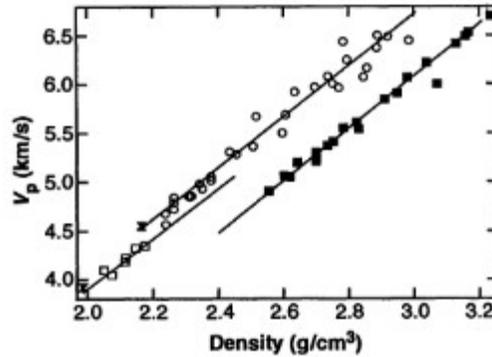
Figure 1: Campbell's et al. P-wave velocity VS sample density results. White circles represent NaCl samples, white squares represent KCl samples and black squares represent KCl samples with CsCl structure developed after the structural change of the KCl samples (Campbell & Heinz, 1992).
