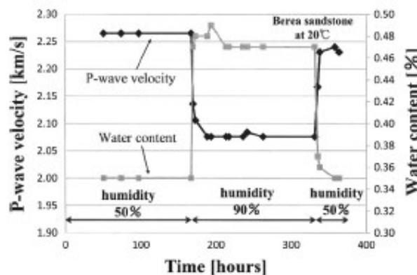
Figure 6: P-wave velocity and water content results for Berea sandstone core experiment with a constant environmental temperature of 20 °C (Nakao et al., 2016)
