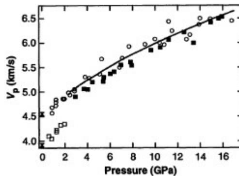
Figure 2: Campbell's et al. P-wave velocity VS external pressure results. White circles represent NaCl samples, white squares represent KCl samples and black squares represent KCl samples with CsCl structure developed after the structural change of the KCl samples (Campbell & Heinz, 1992).
