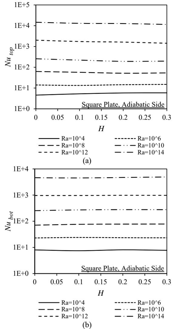
**Fig. 6** Variations of the mean Nusselt number for the (a) top (upper) surface and (b) bottom (lower) surface of a square plate having an adiabatic vertical side surface with dimensionless plate thickness,  $H$ , for various values of the Rayleigh number
