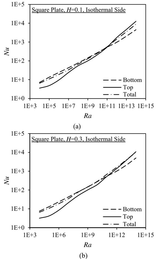
**Fig. 8** Variations of the mean Nusselt numbers for the bottom and top surfaces and for all heated surfaces with Rayleigh number for a square plate having an isothermal vertical side surface for a dimensionless plate thickness,  $H$ , of (a) 0.1 and (b) 0.3
