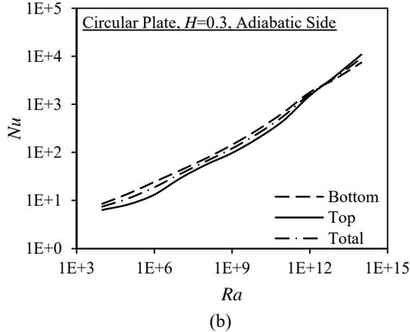
**Fig. 5** Variations of the mean Nusselt numbers for the bottom and top surfaces and for all heated surfaces with Rayleigh number for a circular plate having an adiabatic vertical side surface for a dimensionless plate thickness,  $H$ , of (a) 0.1 and (b) 0.3
