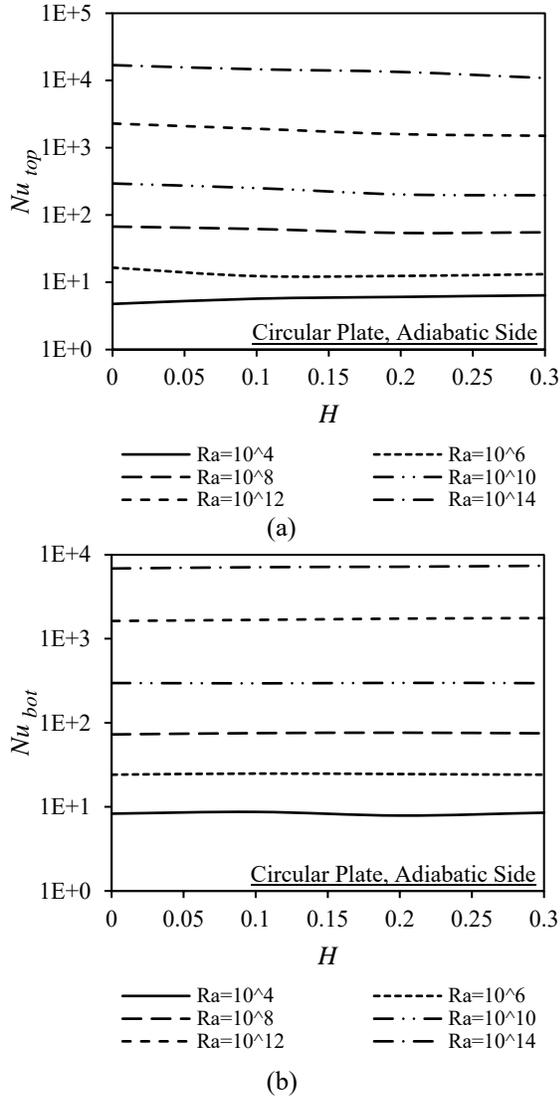
**Fig. 7** Variations of the mean Nusselt number for the (a) top (upper) surface and (b) bottom (lower) surface of a circular plate having an adiabatic vertical side surface with dimensionless plate thickness,  $H$ , for various values of the Rayleigh number
