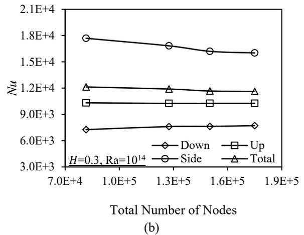
**Fig. 3** Effect of grid number on numerical results at: (a)  $Ra=10^7$  and (b)  $Ra=10^{14}$  for a circular plate having a dimensionless thickness,  $H$ , of 0.3
