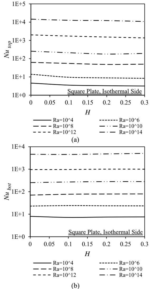
**Fig. 10** Variations of the mean Nusselt number for the (a) top (upper) surface and (b) bottom (lower) surface of a square plate having an isothermal vertical side surface with dimensionless plate thickness,  $H$ , for various values of the Rayleigh number
