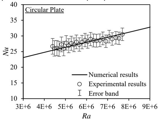
**Fig. 19** Comparison between numerical and experimental results for the circular plate
