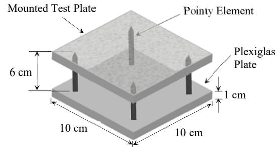
**Fig. 17** Schematic representation of the experimental setup. Shown is the square plate mounted on the support frame.
