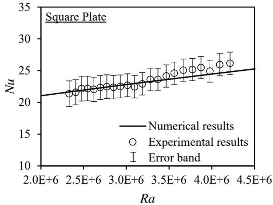
**Fig. 18** Comparison between numerical and experimental results for the square plate
