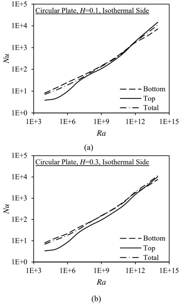
**Fig. 9** Variations of the mean Nusselt numbers for the bottom and top surfaces and for all heated surfaces with Rayleigh number for a circular plate having an isothermal vertical side surface for a dimensionless plate thickness,  $H$ , of (a) 0.1 and (b) 0.3
