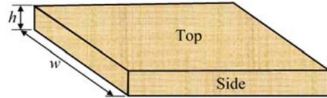
**Fig. 1** Finite thickness plate situation considered, a square plate being shown. Also shown are the definitions of the plate thickness,  $h$ , and of the top (upper) and of the vertical side surface of a two-sided plate. The bottom (lower) surface is below the top surface
