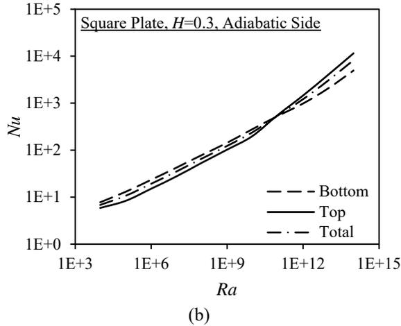
**Fig. 4** Variations of the mean Nusselt numbers for the bottom and top surfaces and for all heated surfaces with Rayleigh number for a square plate having an adiabatic vertical side surface for a dimensionless plate thickness,  $H$ , of (a) 0.1 and (b) 0.3
