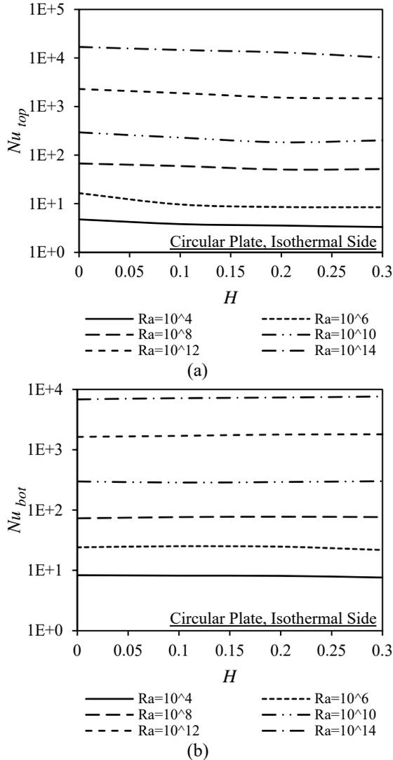
**Fig. 11** Variations of the mean Nusselt number for the (a) top (upper) surface and (b) bottom (lower) surface of a circular plate having an isothermal vertical side surface with dimensionless plate thickness,  $H$ , for various values of the Rayleigh number
