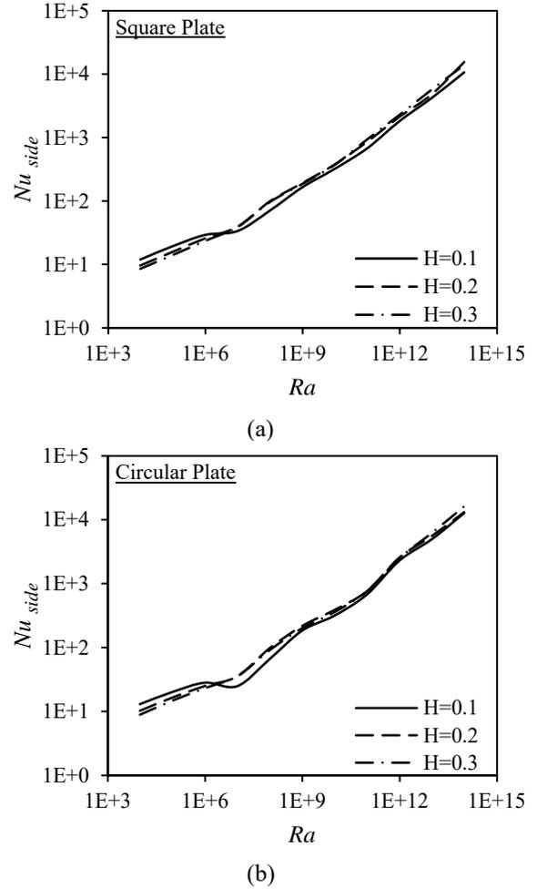
**Fig. 12** Variations of the mean Nusselt number for vertical side surface with Rayleigh number for a (a) square plate and (b) circular plate having an isothermal vertical side surface for dimensionless plate thicknesses,  $H$ , of 0.1, 0.2, and 0.3
