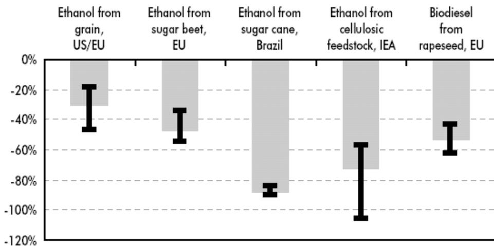
Note: This figure shows reductions in well-to-wheels CO<sub>2</sub>-equivalent GHG emissions per kilometre from various biofuel/feedstock combinations, compared to conventional-fuelled vehicles. Ethanol is compared to gasoline vehicles and biodiesel to diesel vehicles. Blends provide proportional reductions; e.g. a 10% ethanol blend would provide reductions one-tenth those shown here. Vertical black lines indicate range of estimates; see Chapter 3 for discussion.
