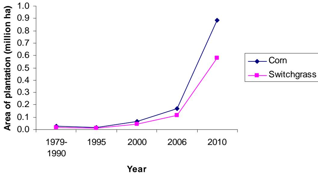
**Fig 5:** Land requirements to meet 5% of transportation fuel derived from corn and switchgrass in Canada
