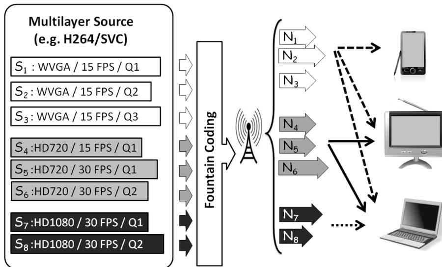
**Figure 5.1:** System setup for the proposed rateless-based video multicast
