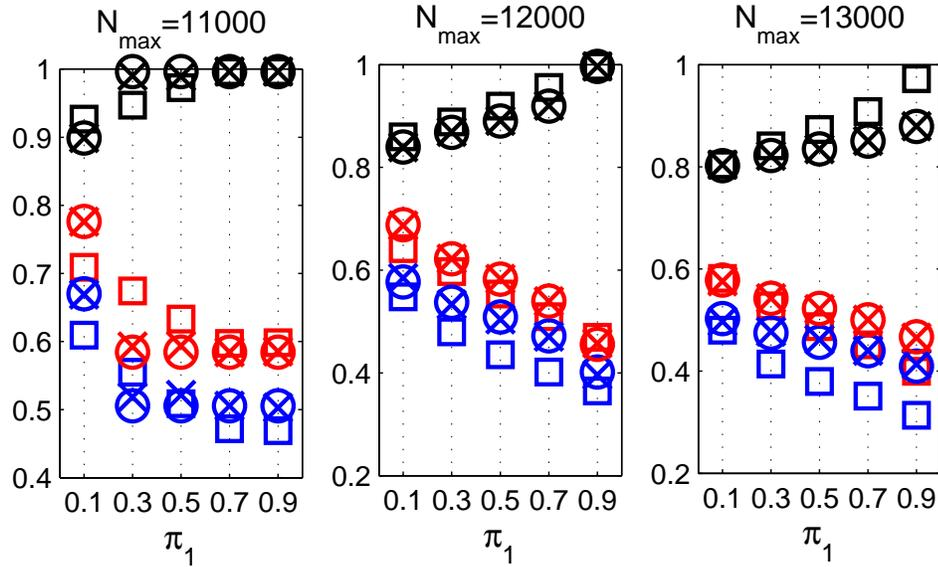
**Figure 5.3:**  $\delta_{min,1}$  (blue) ,  $\delta_{min,2}$  (red) and  $\delta_{min,3}$  (black) obtained using (square) Convex Optimization , (cross) Gradient Descent and (circle) Brute-force search for various settings for prior weights in Table 5.2 ( $\pi_2 = 1 - \pi_1$ ).
