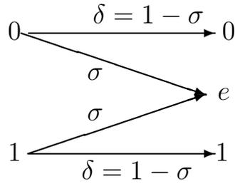
**Figure 2.1:** Binary erasure channel (BEC) with erasure probability  $\sigma$ .
