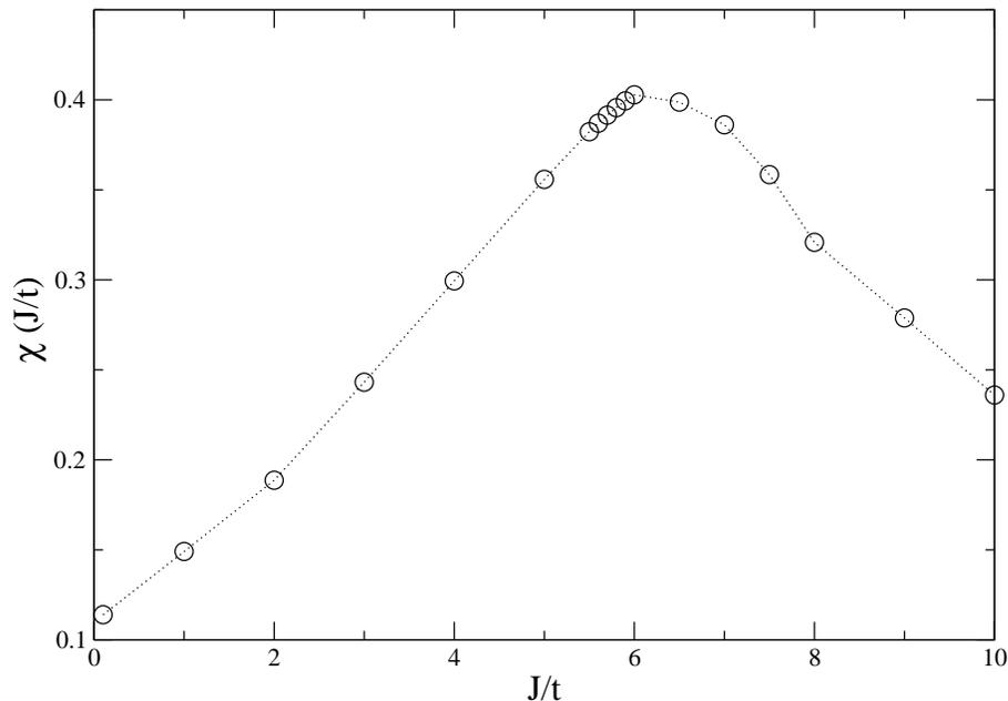
Figure 4.12: Plots of the susceptibilities vs.  $\frac{J}{t}$  for the filling of  $N_e = 4$ . Like the quarter- and sixth-filled one-dimensional chains shown in the last section, this shows a marked rise in susceptibility as  $\frac{J}{t}$  is increased. However, the system does not exhibit the sharp peaks seen in the one-dimensional case, but it is a rather smooth transition through the maximum.
