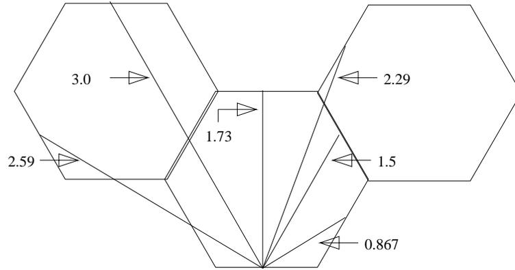
Figure 4.13: The unique nearest-neighbour distances on the  $L = 3$  honeycomb lattice. The sites of the atoms are located on the corners of the hexagons. Note the distances between pairs,  $|\mathbf{r}_{i,j}|$ , are measured from the point in between the sites. Not all of the distances have the same weight as some distances occur more than others. For instance  $|\mathbf{r}_{i,j}| = 2.29$  occurs eight times while  $|\mathbf{r}_{i,j}| = 2.59$  occurs only twice.
