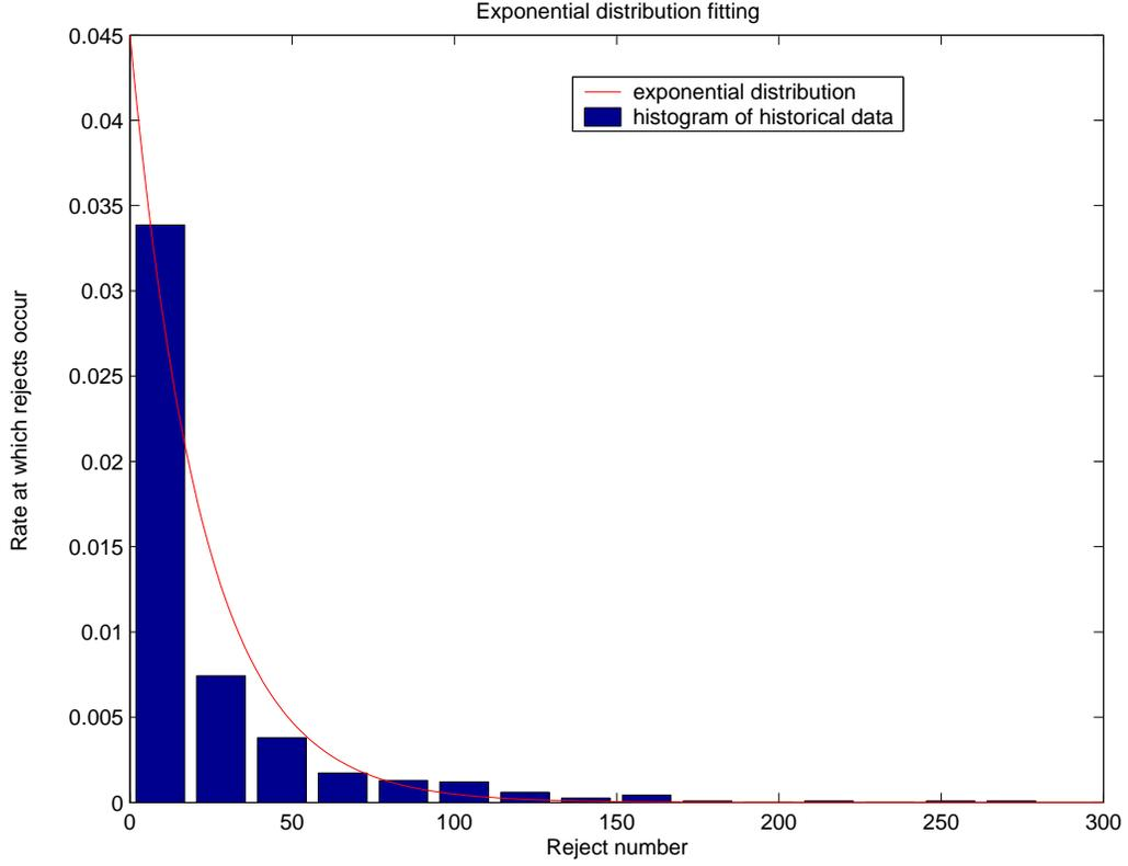
Figure 2.2: Exponential distribution fitting of aggregate occurrences of rejects
