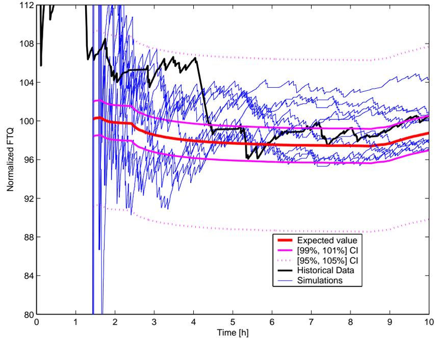
Figure 3.7: Comparison of several FTQ estimations done by the SFM approach and FTQ calculated from the historical data and FTQ expected value
