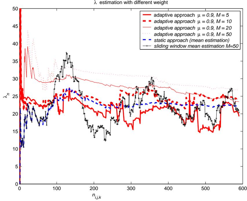
Figure 2.5:  $\lambda$  Estimation for a specific configuration  $(i, j, k)$  as a function of  $n_{i,j,k}$  - comparison for different values of the parameter  $M$
