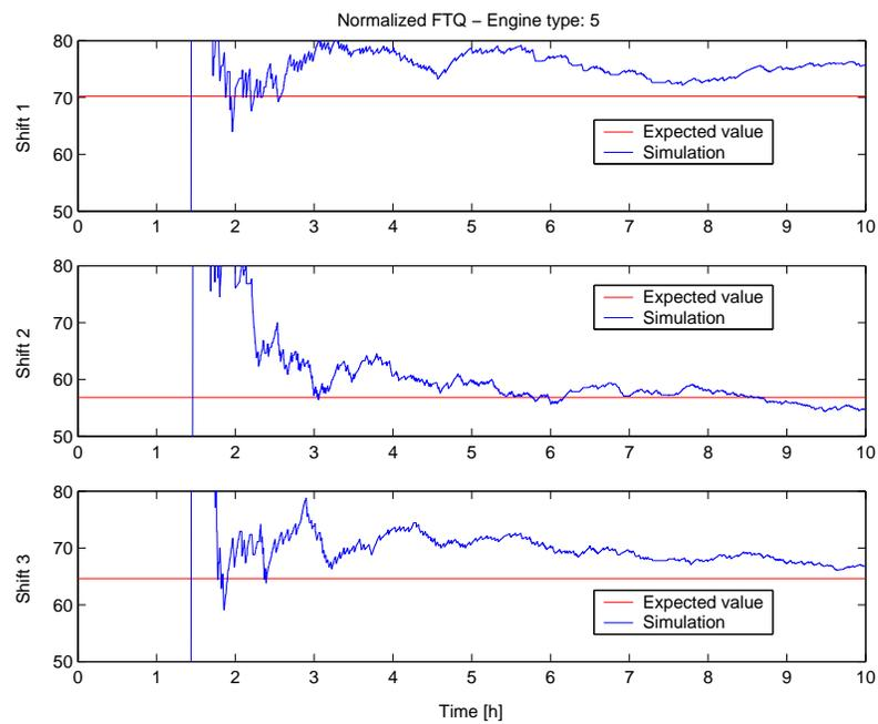
Figure 3.2: Comparison for the three shifts of FTQ estimated by the SFM approach and the expected value for engine type 5
