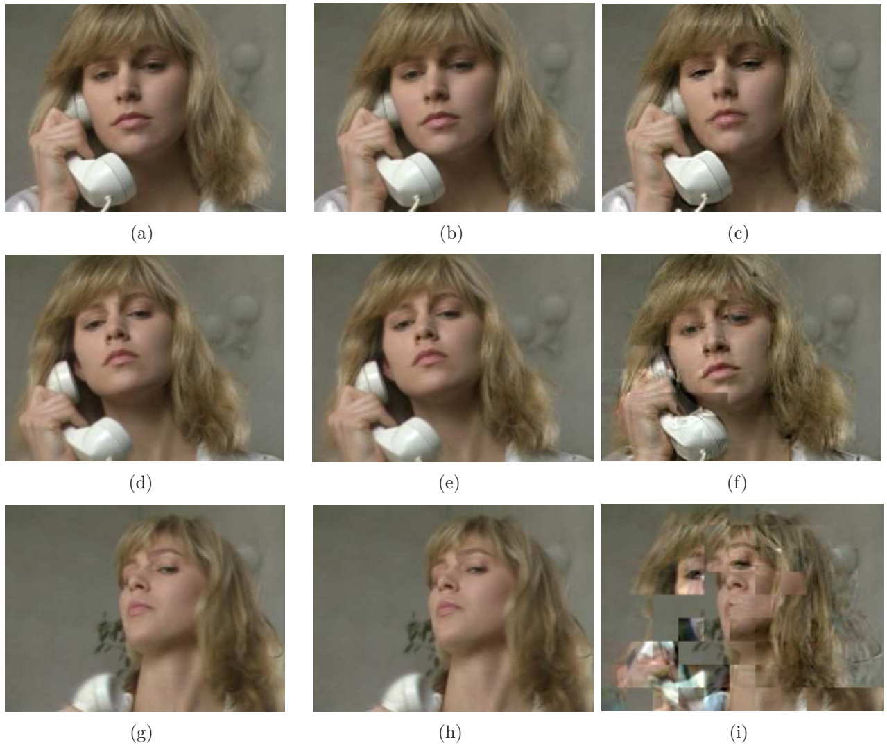
Figure 5.3: Effect of loss of motion vectors and loss of the same amount of prediction error bits on MPEG video Suzie. Frames on the left are the originals, motion vectors of frames on the right are lost, and the same number of prediction error bits in each frame in the middle column is lost too. (a),(b),(c) Frame No. 51. (d),(e),(f) Frame No. 87. (g),(h),(i) Frame No. 107.
