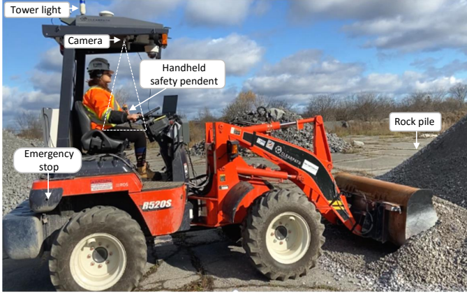
Fig. 4: Kubota R520s wheel loader controlled using hand gestures excavating a rock pile.
