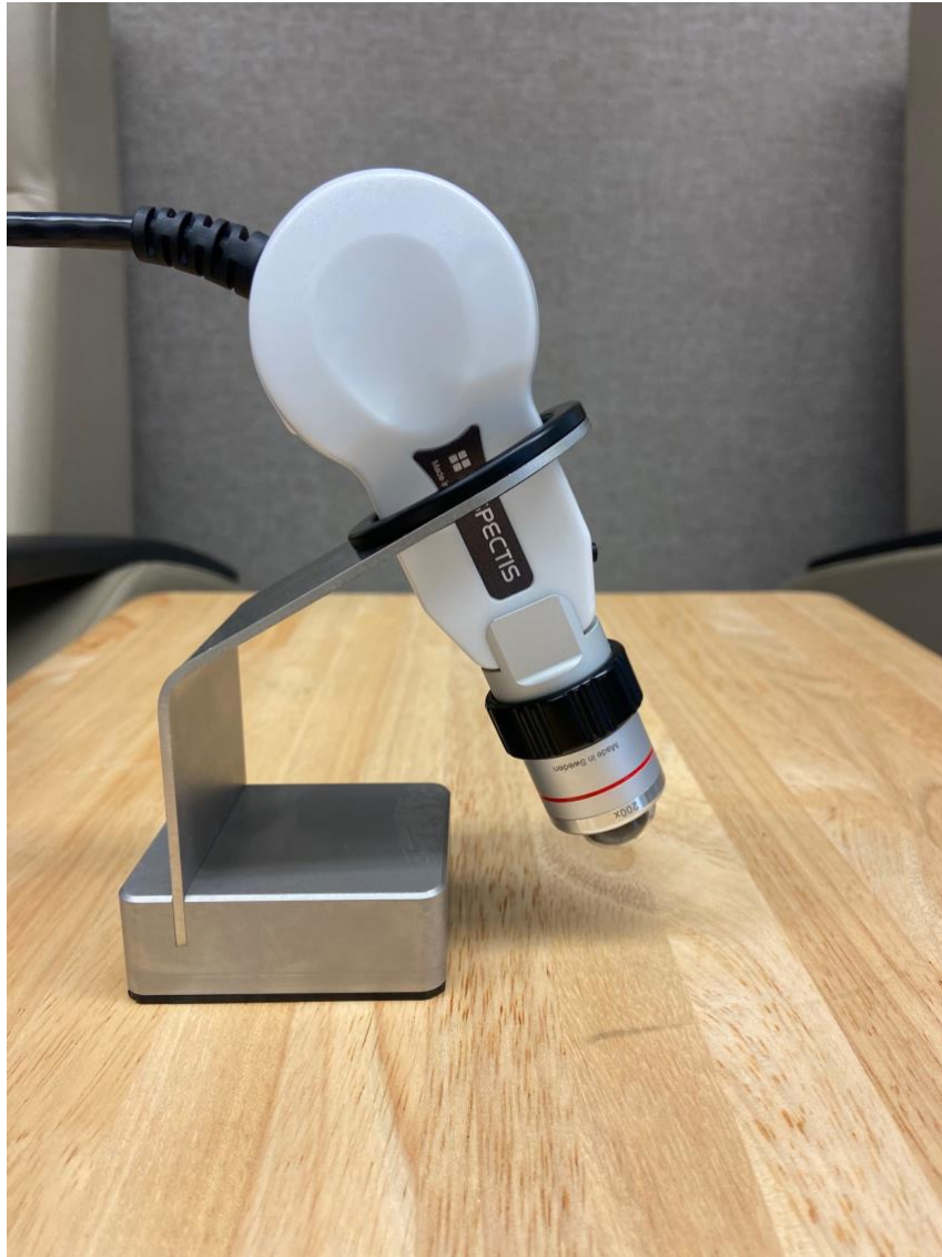
Figure 4: The INSPECTIS Nailfold Video Capillaroscope. This digital capillaroscope has a 5.0MP image resolution and a 200x magnification lens with built-in illumination.
