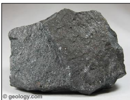
Figure Appendix 60: Typical magnetite specimen exhibiting a gray metallic luster. (Geology.com, 2005-2015)
