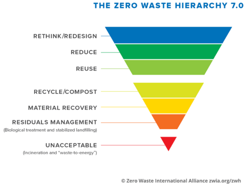
Figure 1: The waste hierarchy, which shows various management options for waste. The most preferable options are at the top. Hospitals may be an institution where one can only go so high. Photo from the Zero Waste Alliance Canada website ( https://zerowastecanada.ca/zero-waste-hierarchy/ )
