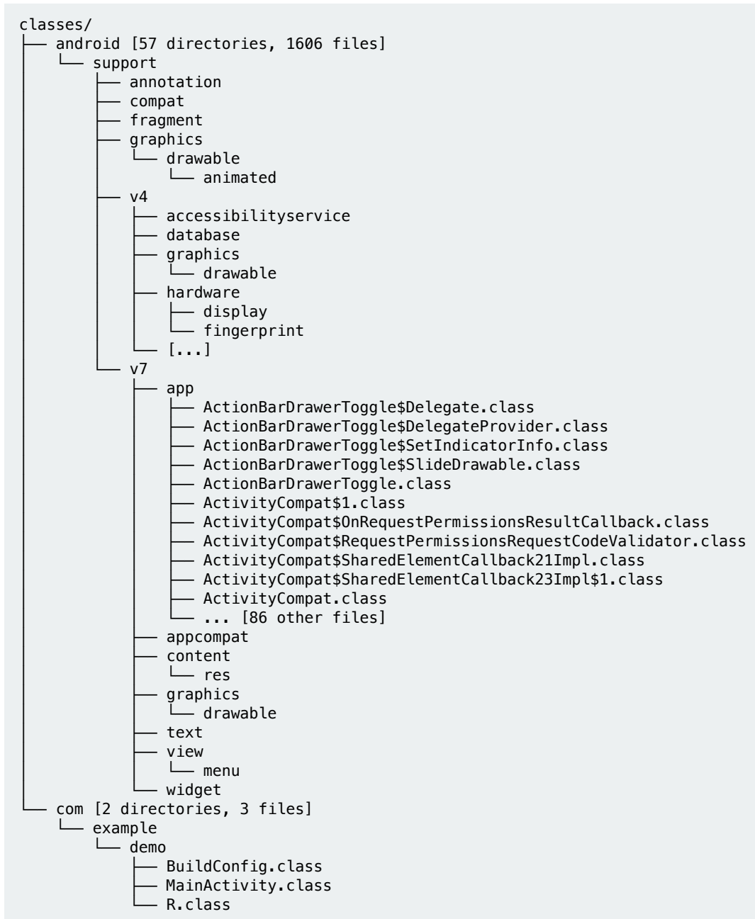
Figure 2.4: Contents of an unobfuscated classes.dex file
