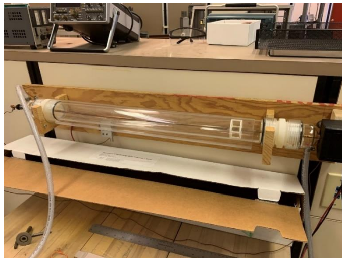
Figure 3: The discharge tube, electrodes, and connections used in the apparatus.
