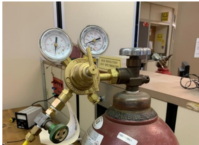
Figure 5: The gas canister along with gauges and connectors used to control the flow of gas into the tube.
