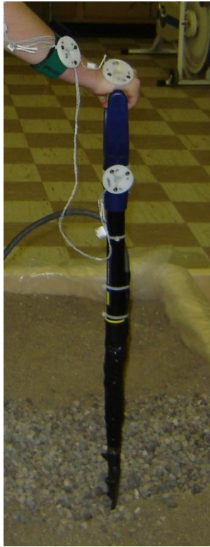
Figure 6-1: Clusters of Infrared Emitting Diodes (IRED) on the right forearm, dorsal surface of the hand, and shovel.
